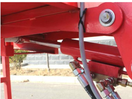
Tilt Angle Sensor,Platform won't Up/Down if body more than 4°
