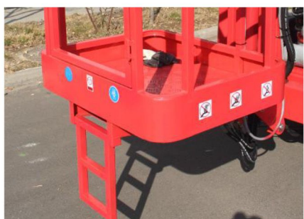
Small Cylinder Under Basket to Keep the Platform Horizontal
