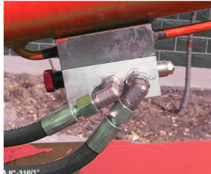
Hydraulic Oil Tank Filtration Alarm System
