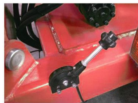
Diesel/Gas Motor are equipped with manual accelerator .
