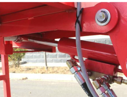
Tilt Angle Sensor,Platform won't Up/Down if body more than 4°
