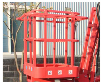
Safety Lock of Basket Prevent Shake when Tow the basket.
