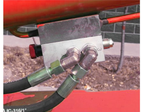
Hydraulic Oil Tank Filtration Alarm System
