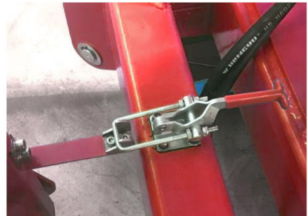
Safety Lock of Arm.Prevent Shake when Tow the Lift
