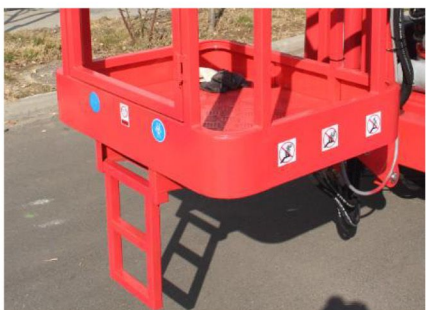
Small Cylinder Under Basket to Keep the Platform Horizontal
