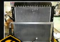
DUAL COOLING SYSTEM
