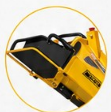
Extended feeding chute, allowing to feed longer branch
