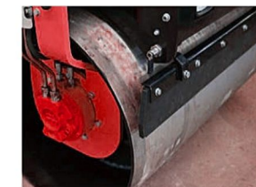
Wear-resistant scraper that can be fully adjusted.
