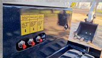
Centralized Grease Bank
