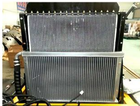
DUAL COOLING SYSTEM
